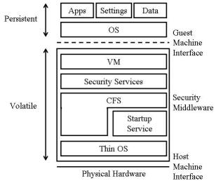
Figure 2. PCSM software architecture
