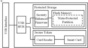
Figure 1. PCSM hardware architecture
