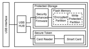
Figure 1: PCSM hardware architecture
