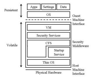
Figure 2: PCSM software architecture
